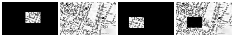
Fig. 3. Example of application of our algorithm to the Image Matching problem. In this case the goal is to find the location of the patch I_{input} in I_{target} . From left to right: I_{input} , I_{target} , the output of the algorithm, the differences between I_{target} and the estimated location of I_{input} in I_{target} . The black box means that the algorithm was able to correctly locate the patch over I_{target} .
